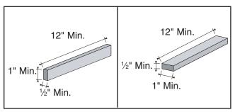
**Figure 27.** Minimum dimensions for edge jointing and surface planing (jointer).
